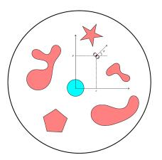
E.g., impossible for this differential drive robot to stably aim within  $\pm 179$  degrees of the origin while "strictly" avoiding obstacles.
